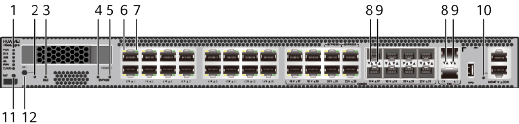
Figure 3-55 Indicators and buttons on the USG6575E-B
